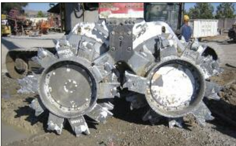
Figure 6 – CSM: A marriage of soil mixing technology with hydro-fraise equipment.
