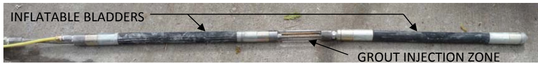
FIG. 5: Typical Straddle Packer
