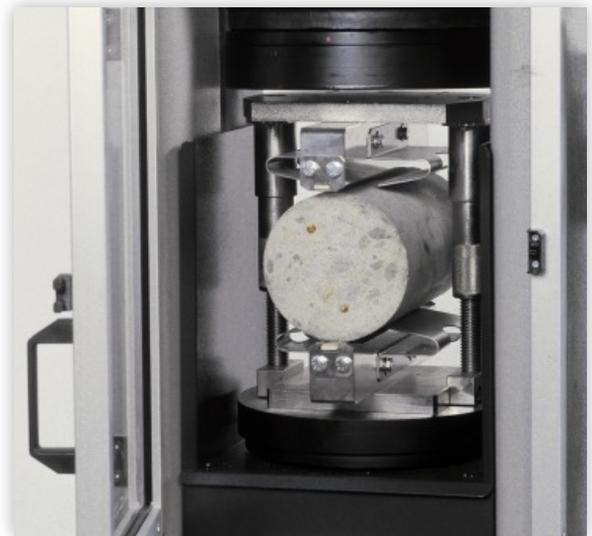
Figure 7. ASTM C469 Concrete Cylinder Tensile Testing Apparatus
