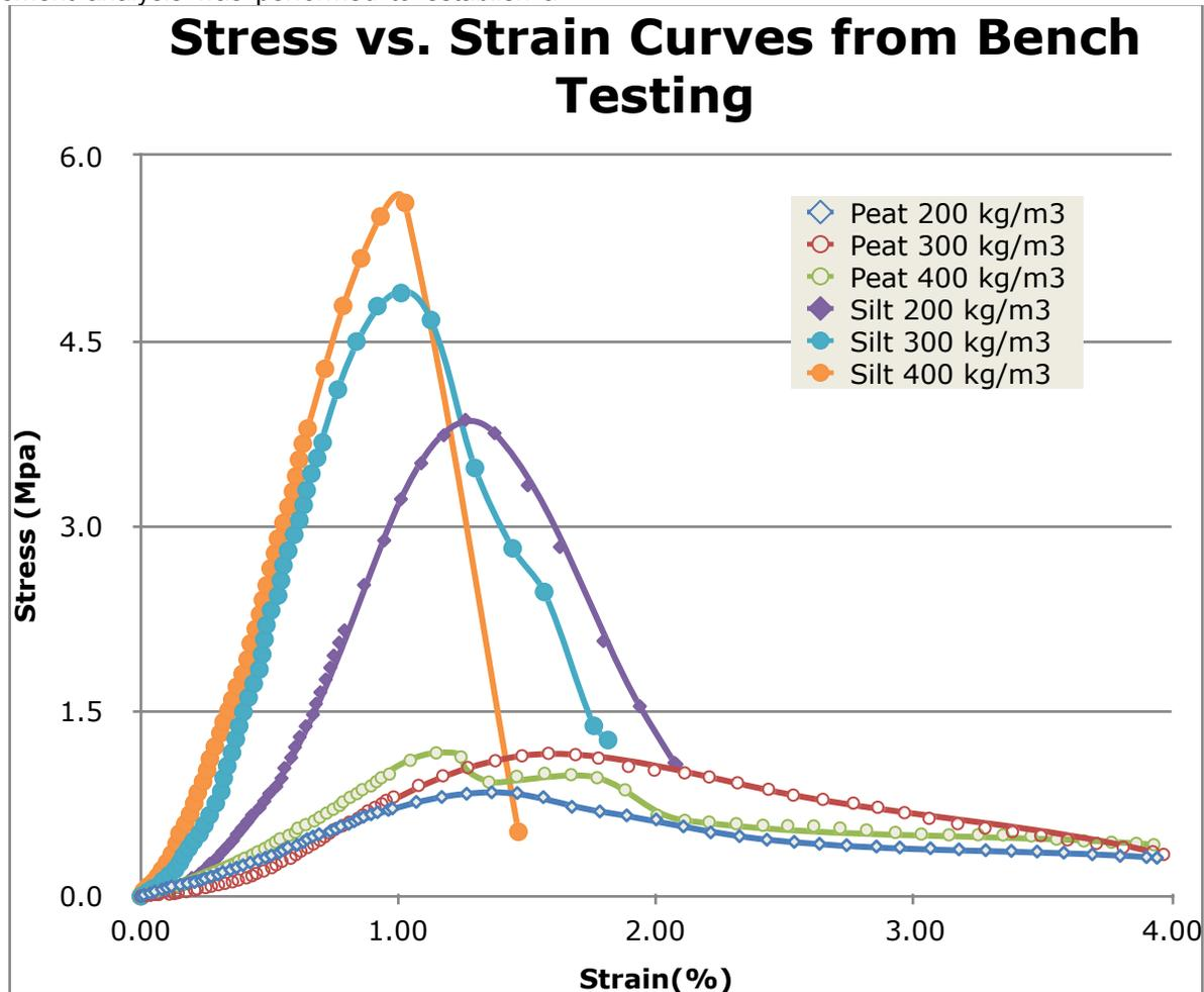
Figure 1. Bench Test Soil-Cement Compressive Stress-Strain Behavior
