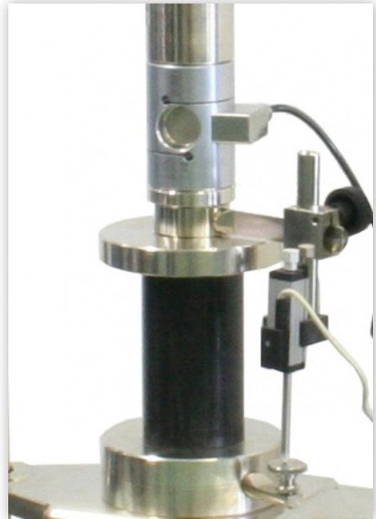
Figure 2. ASTM C39 Modulus Determination
