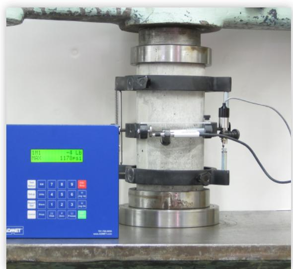
Figure 3. ASTM C469 Modulus Determination
