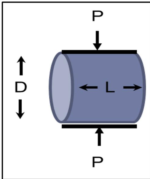
Figure 6 – Illustration of Splitting Test
